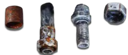
Competitor A after 1,000 hours ASTM B117 (ISO 9227) salt spray test
